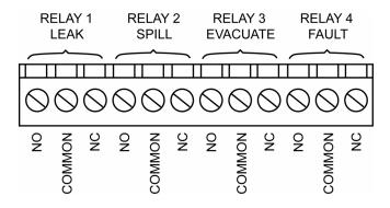
Each relay may be connected as normally open (NO), or normally closed (NC).
